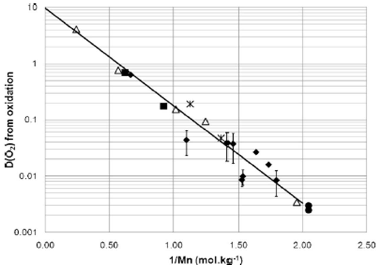
Effect of avg. mol. Wt. of carrier blend on O<sub>2</sub> diffusion rate.
