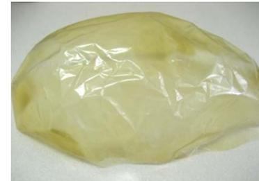
Zein nanoclay nanocomposite films were fabricated at different nanoclay contents using two methods: solvent casting and extrusion blowing methods.
