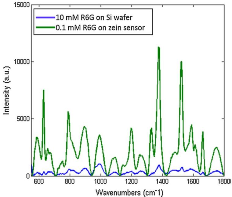
The effect of gold-coated inverted pyramid zein platform on the intensity of the Raman peaks. Enhancement factor (EF) for this platform is  $1.3 \times 10^4$ , and this factor is similar to the original substrate which was used to prepare the platform.
