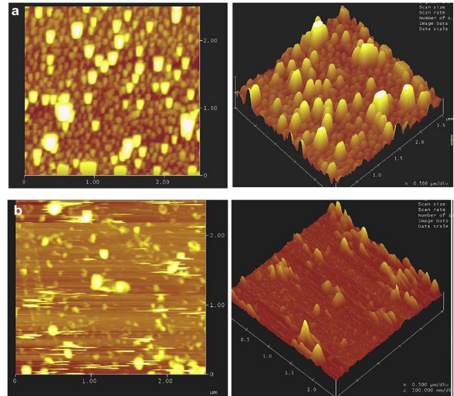
. Fraction 1 (a) and fraction 2 (b) (0.1% in 70% ethanol) as imaged by the AFM; top view (left), 3D view (right), scan size=2.5 mm, data scale=100 nm (Panchapakesan et al. 2012).
