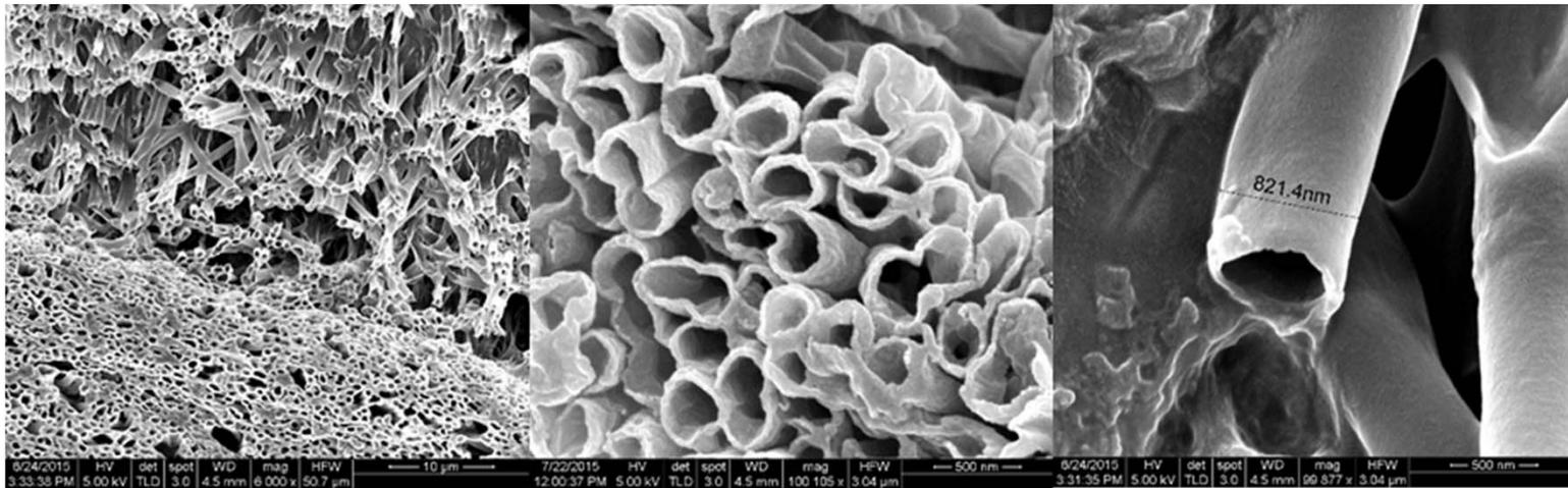
Layer-by-layer fabrication of GRAS nanotubes include alginate and BSA on polycarbonate template. SEM images of alginate/BSA nanotubes with diameter of 800 nm (left and right), and 400 nm (center) (Maldonado et al., 2017)
