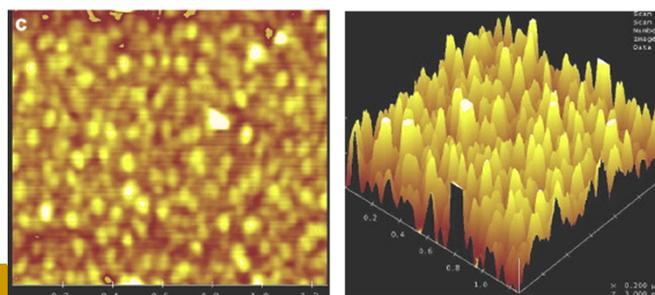
zein film spin cast on a silicon wafer.
