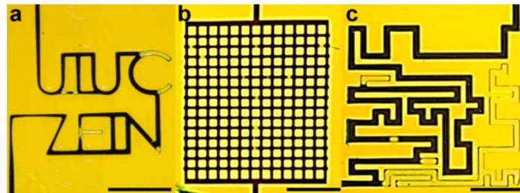
Visualization of zein-glass microfluidic devices with complex fluidic pathways. (a) Interconnected letters composed of continuous microfluidic channels, (b) a microfluidic network with channels and chambers, (c) a solved microfluidic maize maze with multiple false paths. Blue food dye was used for visual aid. All scale bars are 5 mm.
