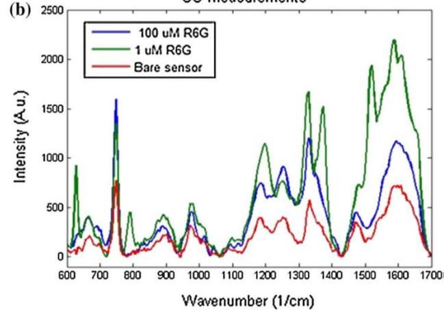
Zein biosensor with nanopores - Rhodamine 6G measurements
