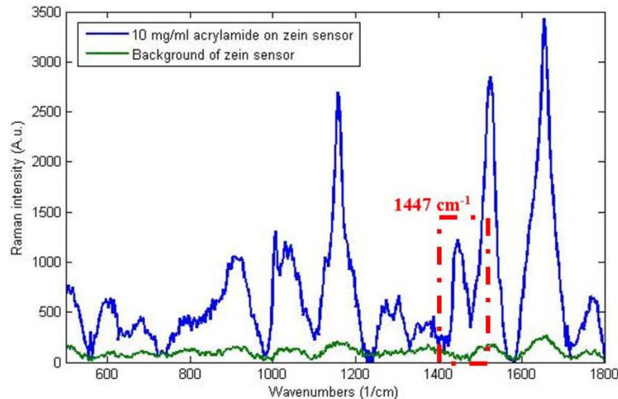
Comparison of the background signature of zein-SERS sensor (green) with acrylamide on top of the sensor (blue). Red dotted square indicates the peak at the wavenumber of 1447 cm<sup>-1</sup>, which does not exist in the background, but exists in acrylamide signature. (A.u.: arbitrary units) (Gizer et al., 2016c).
