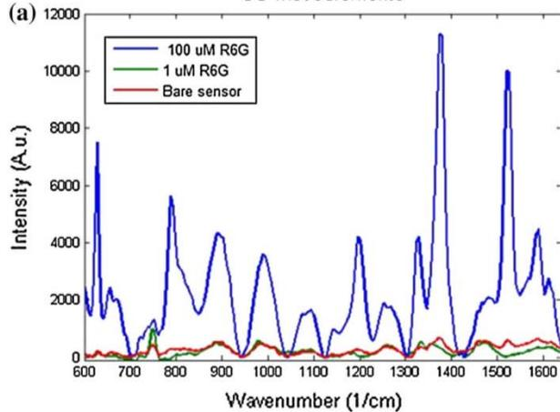
Zein biosensor with nanopillars - Rhodamine 6G measurements
