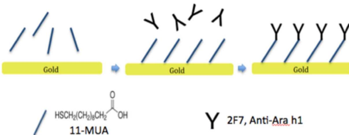
Schematic illustration of the functionalization of the gold surface (Gezer, Liu, Kokini, 2016).
