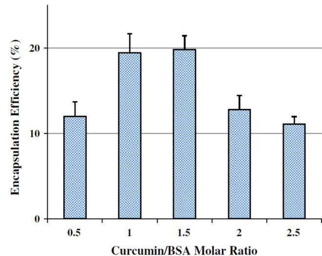
Encapsulation efficiency of curcumin-loaded BSA NPs with the use of ethanol as a desolvating agent (Sadeghi et al. 2014).
