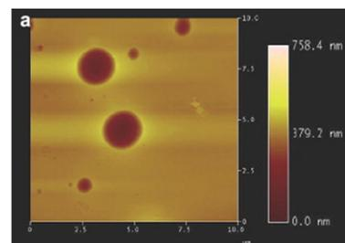
zein film cast from solution on a petri dish
