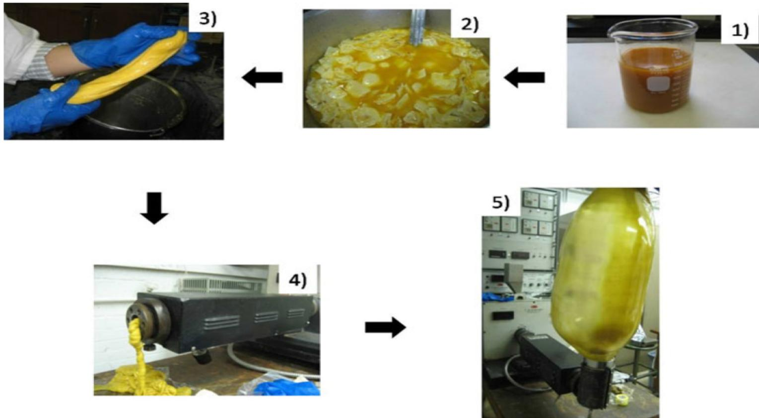
The steps of the blown extrusion technique including 1 zein MMT solution, 2 precipitation, 3 resin formation, 4 cold extrusion, and 5 balloon formation (Luecha, Sozer, and Kokini, 2010).
