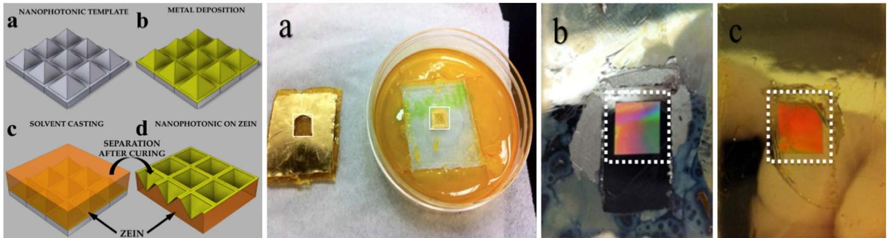
Left: direct transfer of three dimensional metallic nanophotonic structures onto zein (a) is deposited with 200 nanometers of noble metal using E-Beam Evaporation (b). Zein solution is solvent-casted over the metal-coated template (c), and after fully solidifying; the zein film with three-dimensional metallic nanophotonic structures is separated from the template (d).
