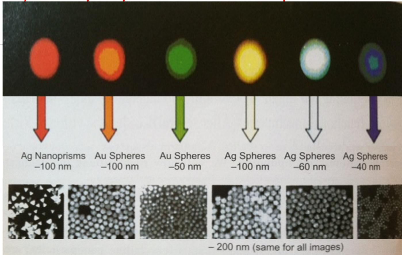
Optical properties of the nanoparticles can be changed with different size, shapes and composition of metal nanoparticle.
