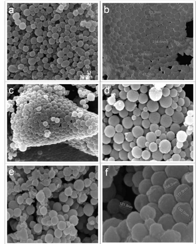
The SEM images of  $\alpha$ -LA nanoparticles (a, b- prepared with ethanol; c, d- prepared with acetone; e, f- prepared with methanol; all in 1:5 water: desolvating agent ratio) (Abdunnasir, 2016).
