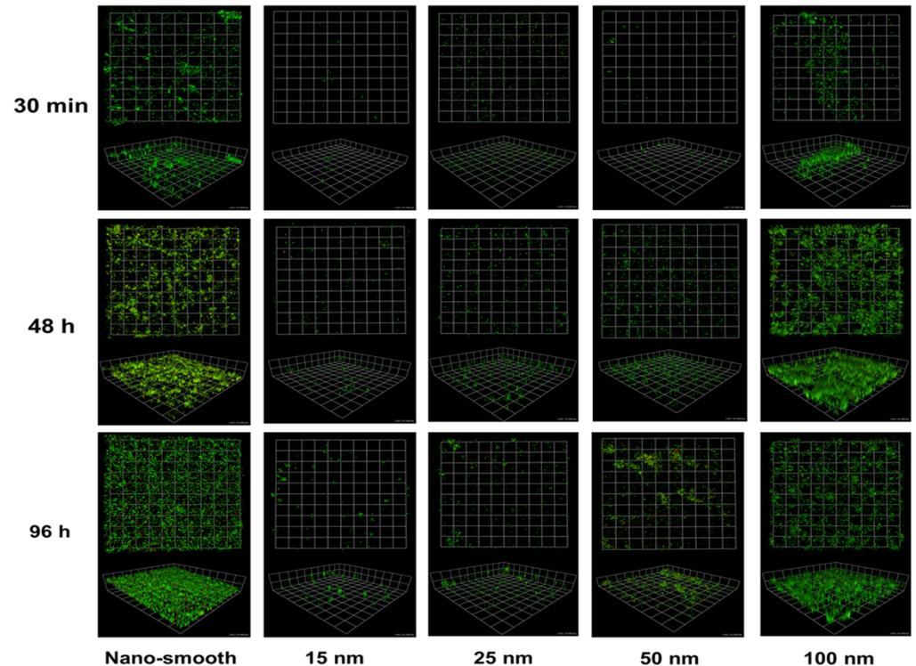
Attachment and biofilm formation by *E. coli* ATCC 25922 at 30 min, 48 h and 96 h on nano-smooth alumina (control) and anodized surfaces of 15 nm, 25 nm, 50 nm and 100 nm pore diameter. (Feng et al., 2014).
