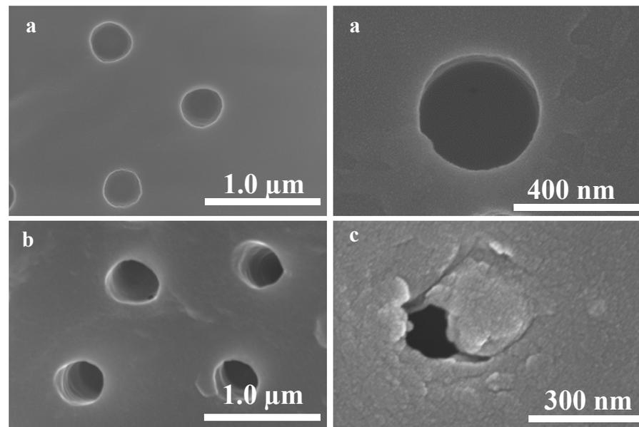
SEM images of one (a), two (b), and three (c) bilayers of PDL (poly-D-Lysine) and BSA (Bovine Serum Albumin) on the surface of PC template, before cleaning
