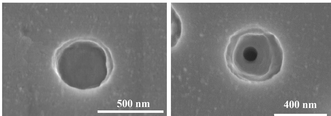
**SEM images of deposition of three bilayers of PDL and BSA
