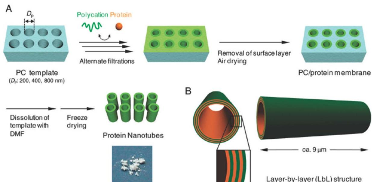
**Synthesis of protein nanotubes by LbL deposition technique using nanoporous PC membrane, Qu and Komatsu, 2010.**
