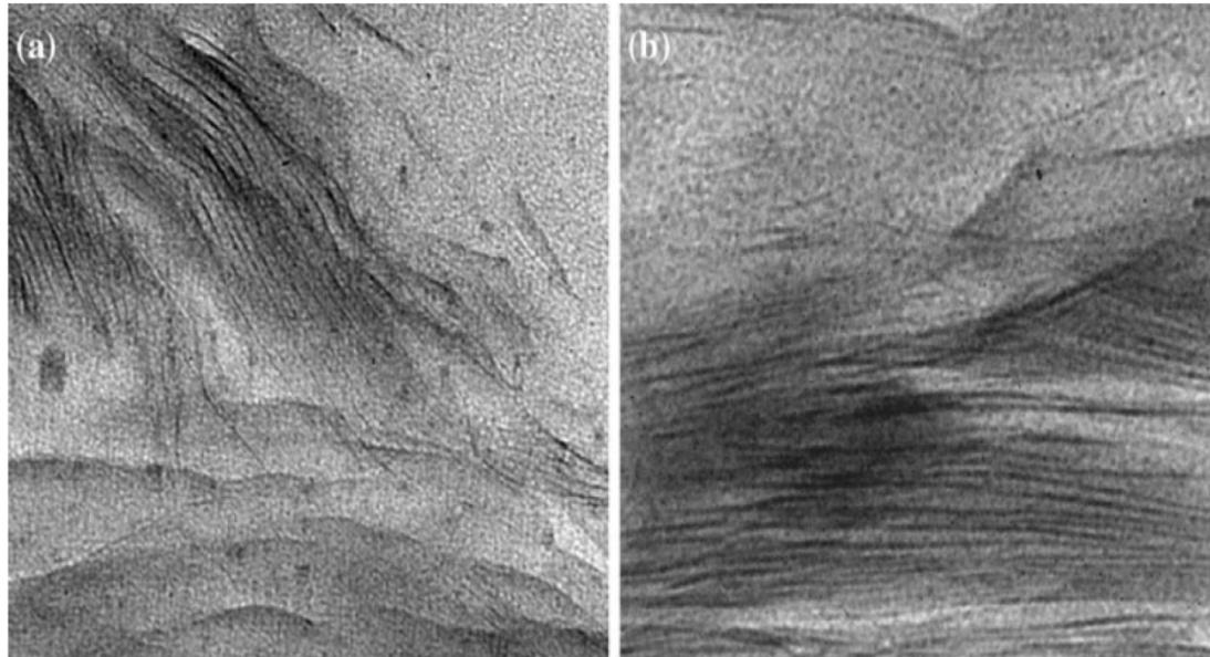
TEM images of a solvent cast zein MMT nanocomposite films with 5 wt% of MMT, and b blown extrusion zein MMT nanocomposite films with 5 wt% of MMT (Luecha, Sozer, and Kokini, 2010).
