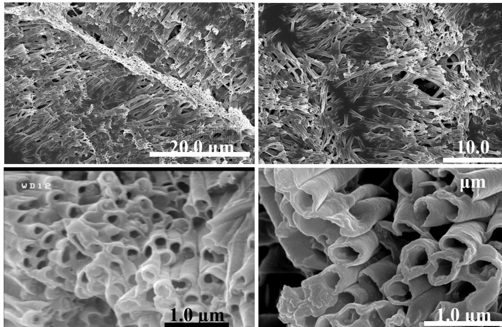
SEM images of (PDL/BSA)<sub>3</sub> bio-nanotubes
