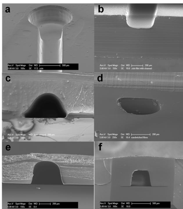
Zein film can accurately replicate the microfluidic features
