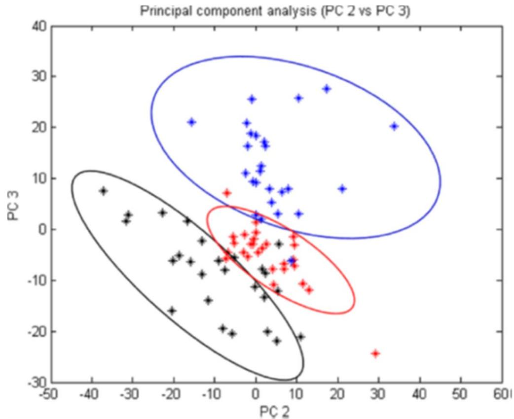
Principal component analysis (PC2 vs PC3) of baseline-corrected Raman spectra for background zein-SERS sensor (black), antibody-functionalized zein-SERS sensor (blue) and Ara h1 protein captured by antibody-functionalized zein-SERS sensor (red) (Gizer, Liu, Kokini, 2016).
