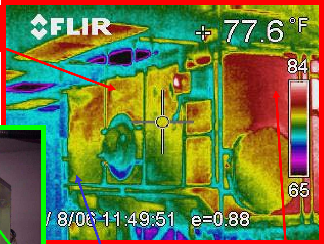
Thermal Image of a Vapor Phase Hydrogen Peroxide Cycle (Poor Distribution)
